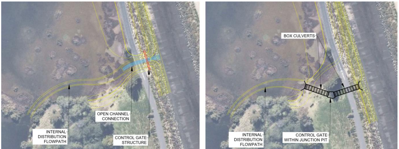
Figure 25 Indicative preliminary options for new inlet structure
