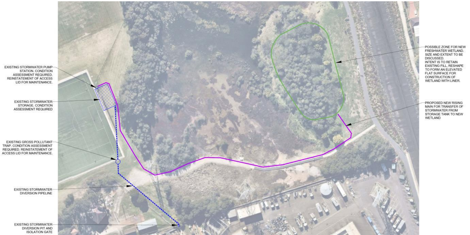
Figure 40 Indicative plan for new constructed wetland
